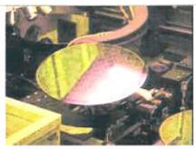
Unlike most forms of manufacturing, which combines a series of discrete components manufactured individually, making a chip entails building up the individual circuit patterns in layers. This involves a variety of processes in which portions of conducting and nonconducting compounds are repeatedly added and stripped away.
