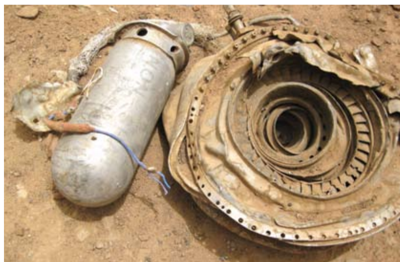
The remains of a Tomahawk missile engine.
