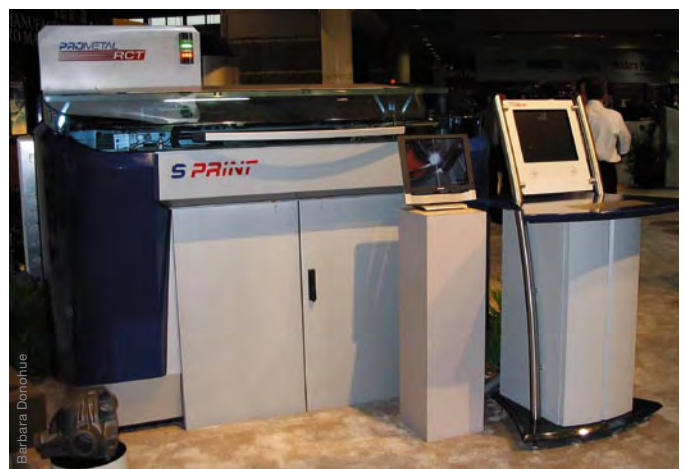
Ex One rapid casting machine creating a sand mould by 3-D printing.
