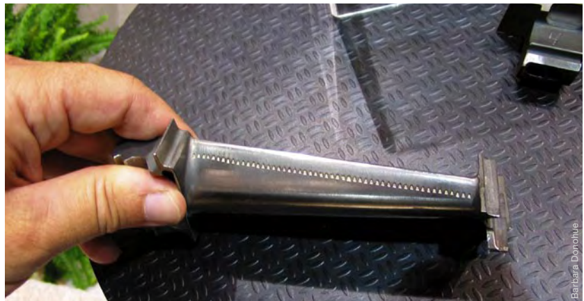
Cooling holes in a turbine blade, an example of laser machining by the Super Pulse technology from Ex One.
