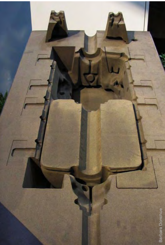
Example of a sand mould built by an Ex One rapid casting machine.
