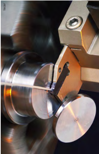
The Jet Cut parting insert from Iscar provides coolant directly to the cutting area through an internal passage.
