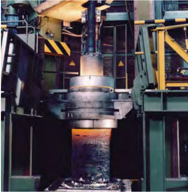
Electro-slag remelt (ESR), showing an ingot in the process of remelting. (Photo courtesy of SCHMOLZ + BICKENBACH.)
