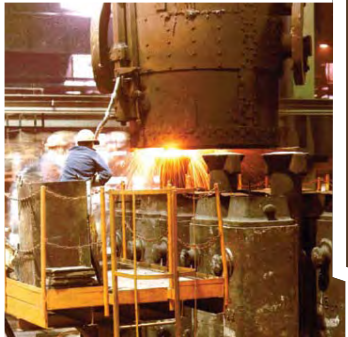
Bottom pouring of tool steel into ingots. (Photo courtesy of SCHMOLZ + BICKENBACH.)
