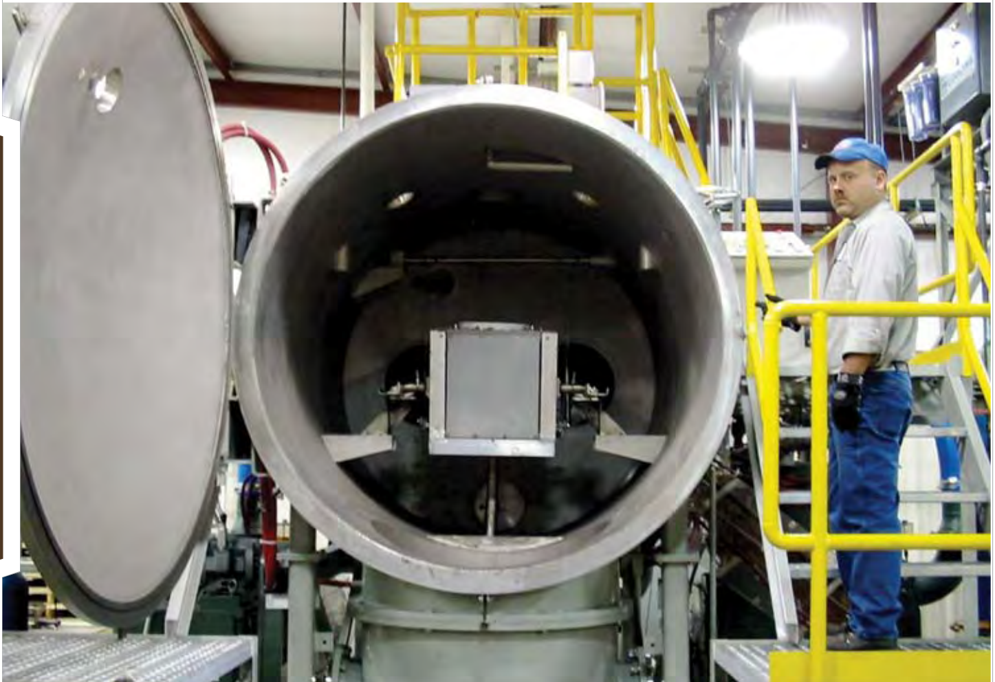
Inside view of vacuum induction melting chamber showing melt coil and crucible. (Photo courtesy of Sophisticated Alloys, Inc.)
